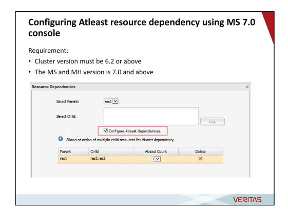
Veritas InfoScale Operations Manager 7.0 provides the functionality of **Atleast Count dependency** where the parent resource depends on a set of child resources. Atleast count dependency can be configured by checking an option while configuring resource dependency. This option is available only if the cluster version is 6.2 or above and the MH version is 7.0 and above.
