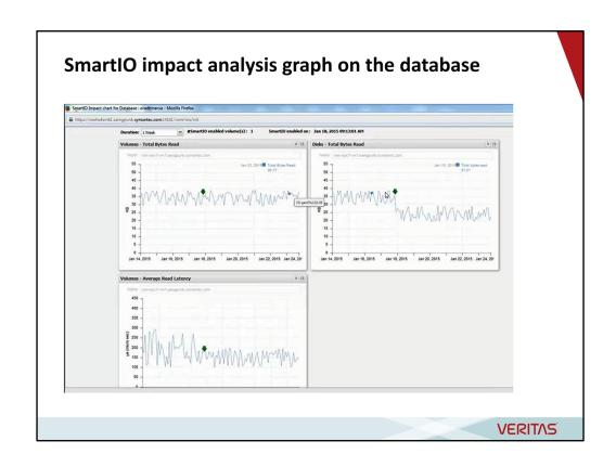
The **Volumes** chart shows reads for the SmartIO enabled volumes on the database. The **Disks** chart shows reads from the disks of the SmartIO enabled volumes. When SmartIO is enabled, reads are served from the SmartIO cache, and hence the number of reads from the disk reduce.
