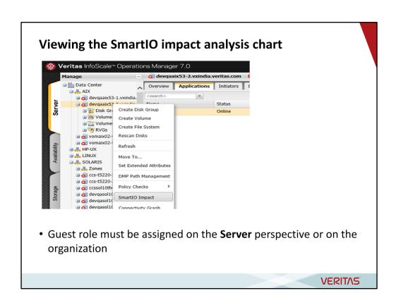
To view the SmartIO impact analysis graph, go to the **Server** perspective and expand **Manage** in the left pane. Right-click the database or the host and select **SmartIO impact**.
