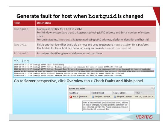
In Operations Manager, a host is uniquely identified using **hostguid**. The **hostguid** is generated using MAC address. So if the MAC address of a host changes the **hostguid** for that host also changes.
