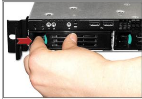
Figure 3-1 Removing a disk drive module
