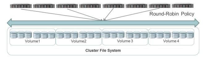
For write scalability we can see how we have a clear linear gain in scalability when using the locality policy, and almost linear when using round robin. When using 16 nodes, the architecture is able to obtain 14.27 GB/s for writes while maintaining two copies of the data for resiliency.
