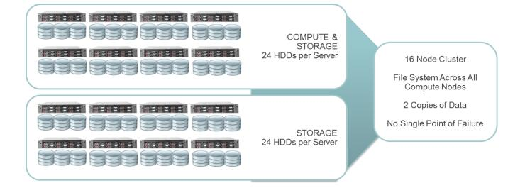
Although all the storage used is internal, Veritas' Flexible Storage Sharing technology, a part of the Veritas InfoScale Storage product, allows the use of SAN storage connected to any of the nodes if greater capacity is needed or to re-use some hardware already available. In the reference architecture discussed here there is no external storage. All the nodes are connected using one InfiniBand switch.
