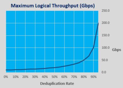
How fast can deduplicated data can be pumped into a 10 Gbps link
